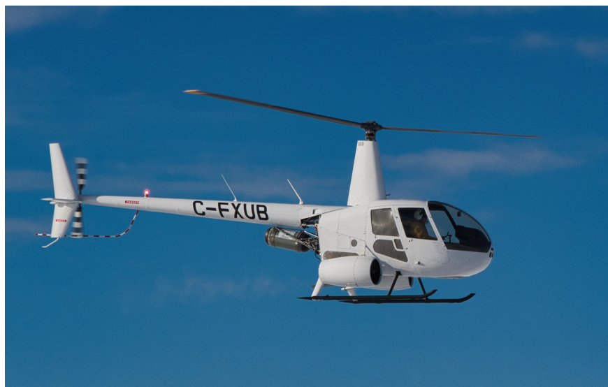
Figure 1. Forward flight tests of the Unither Bioelectronics hydrogen-electric R44 helicopter. The first crewed hydrogen powered fuel cell helicopter.
