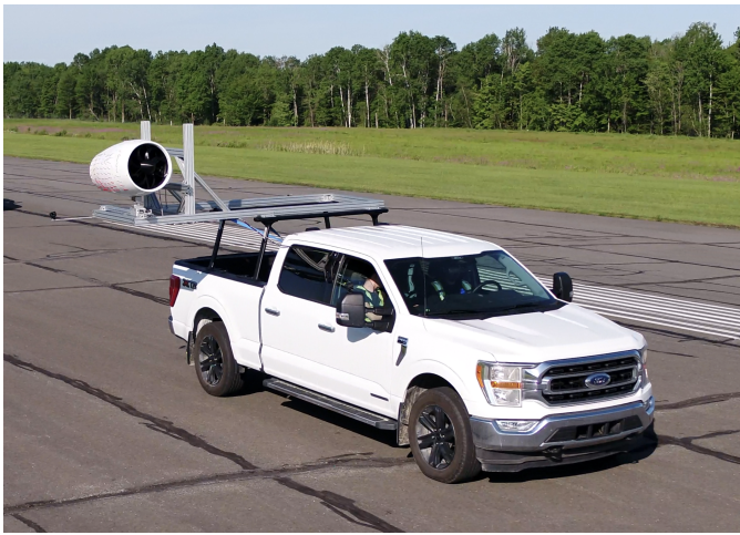
Figure 15. A single radiator nacelle being truck-tested on the runway.
